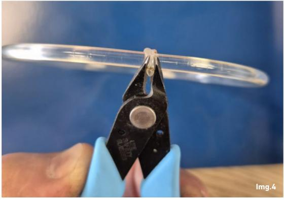
**Note:** If you are having bands fail around the weld, check you have followed the above instructions correctly. If other parts of the band are failing (wearing flat spots, stretching etc.), please check our Tranzband Maintenance & Repair Guide.
